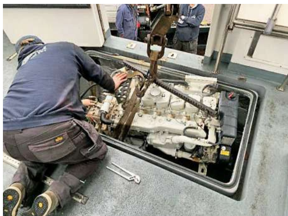
Port engine being removed
