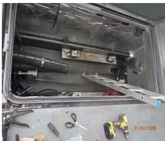
With the old engines removed we took the opportunity to clean and re-insulate the engine spaces. We also modified the fire suppression and battery charging systems. New stern seals, fuel lines and control cables were also installed.
