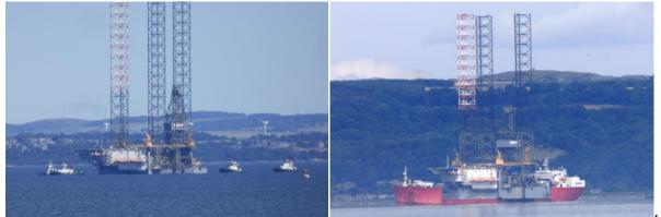
RAN [IMO 8771320], 15,136 gt, Magni Drilling Limited, built 2013 as Hercules Triumph and renamed 2017, is a KFELS Super A class rig designed for harsh environments, able to operate in a water depth of 400ft, maximum drilling depth 35,000ft, with three 525 foot long legs.
